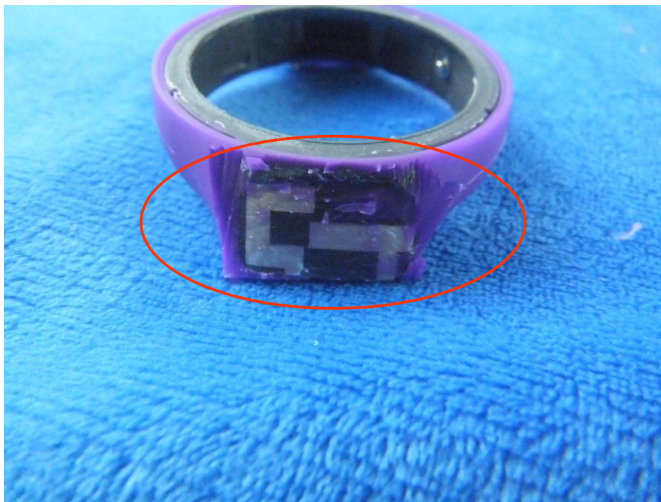
GSM/PCS/UMTS-FDD Antenna View
