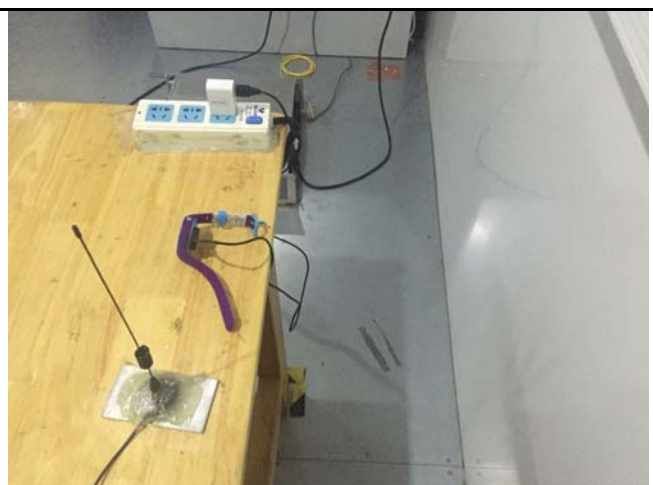
Conducted Emissions Test Setup Side View
