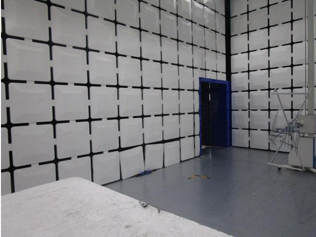
Description: Radiated Spurious Emission Test Setup
