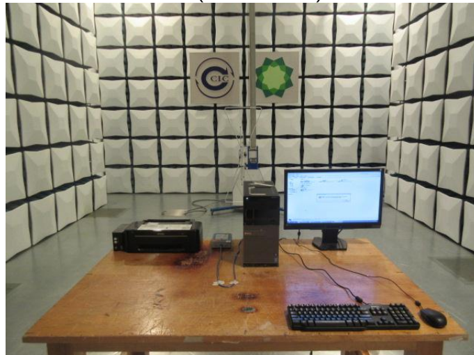
Radiated Emission (30MHz-1GHz) Connect to PC
