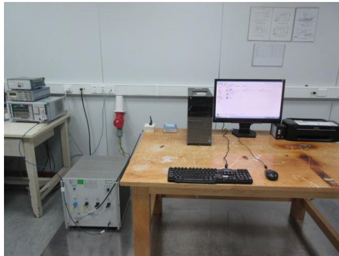
Radiated Emission (30MHz-1GHz) Connect to PC
