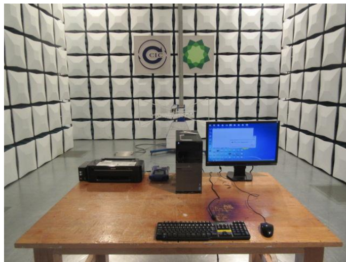
Radiated Emission (above 1GHz) Connect to PC
