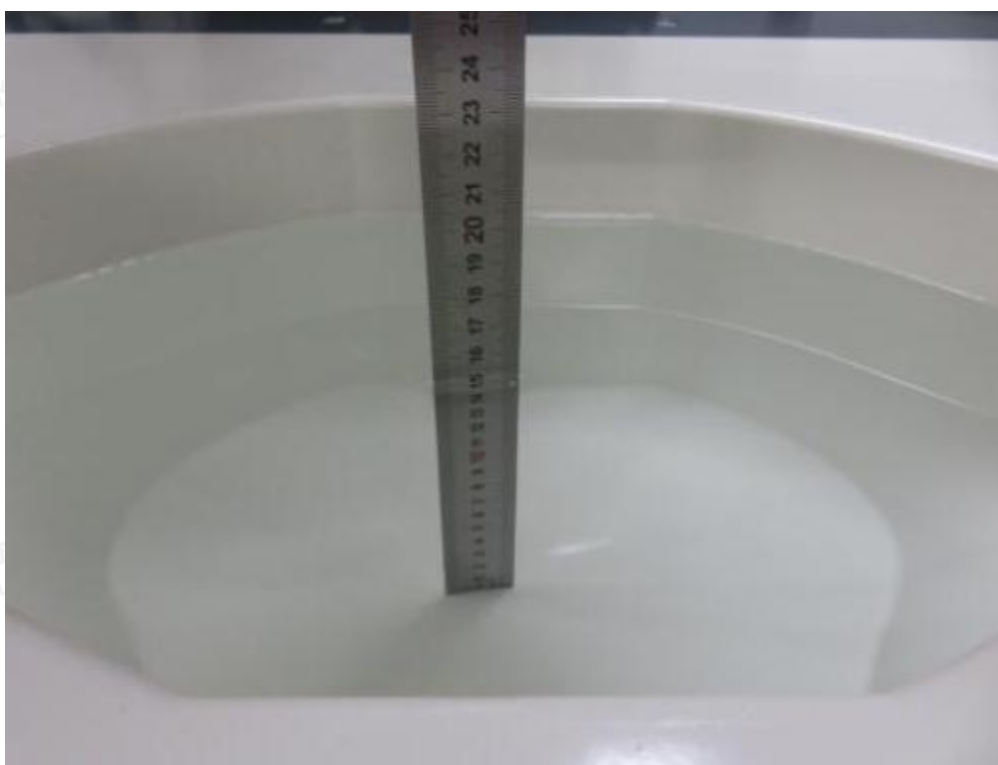
Photograph of the depth in the Head Phantom (2600MHz, 15.5cm depth)
