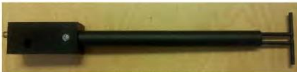
Figure 1 – MVG COMOSAR Validation Dipole
