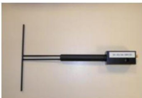
Figure 1 – Satimo COMOSAR Validation Dipole
