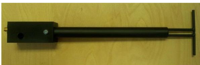
Figure 1 – MVG COMOSAR Validation Dipole
