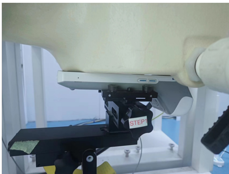
Handheld Front Setup Photo(0 mm)
