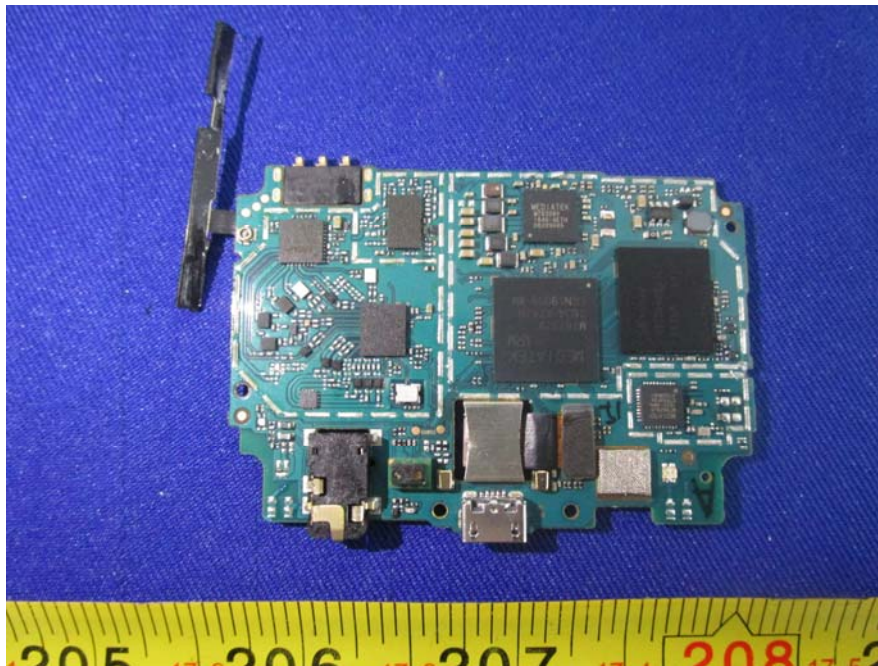
EUT – Mainboard Top View
