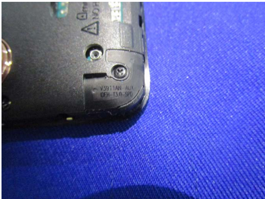
EUT – LTE-DRX Antenna View
