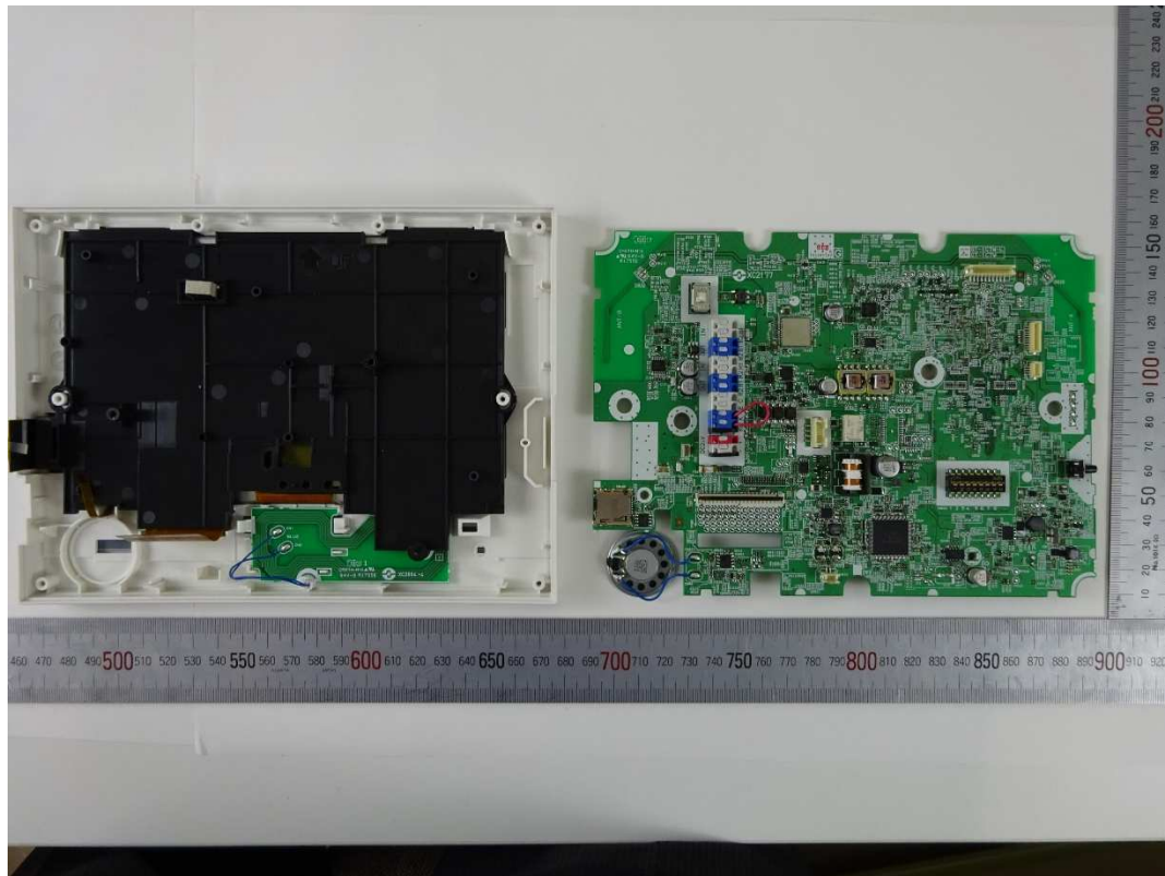
Internal Photos of GT-1C7W-L V2
