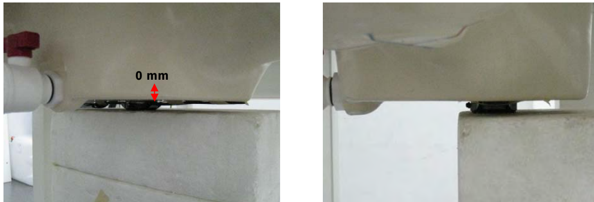
Fig.3 EUT Back side to flat phantom
