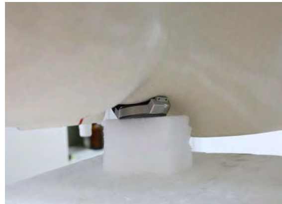
Fig.5 Configuration 3: remove the one side's watchband and make the watch's back touch against the neck phantom area
