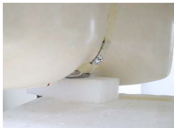
Fig.4 Configuration 2: watch's back touch against the neck phantom area (gap:0mm)
