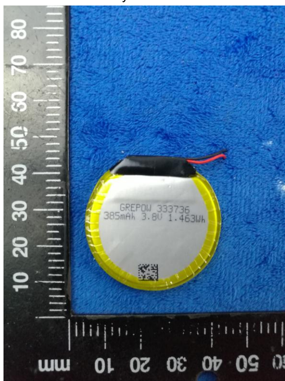
Battery - Front View
