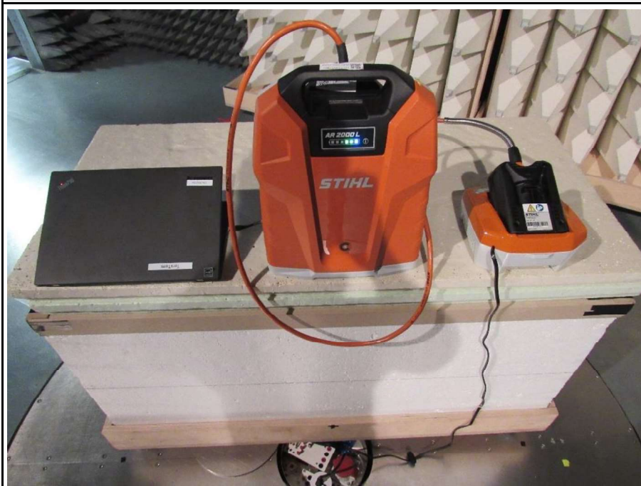
EUT test setup below 1 GHz
