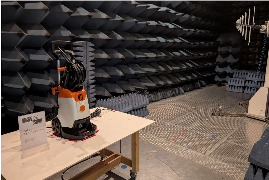
Pre-test setup – SAC [30 – 1000 MHz]
