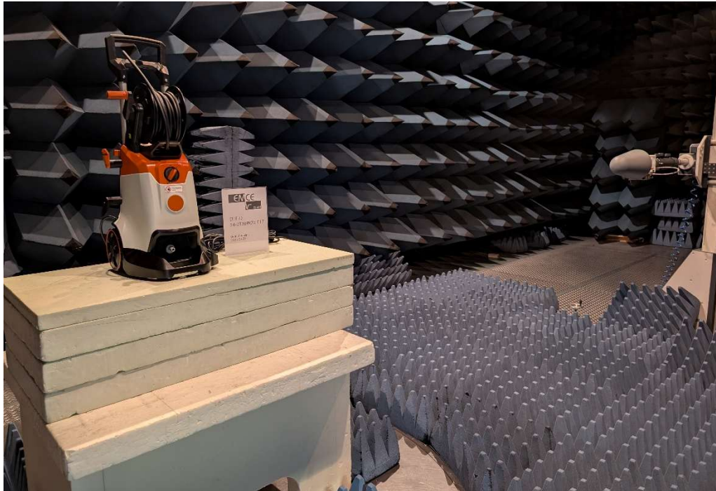
Final test setup – SAC [1 – 10 GHz]
