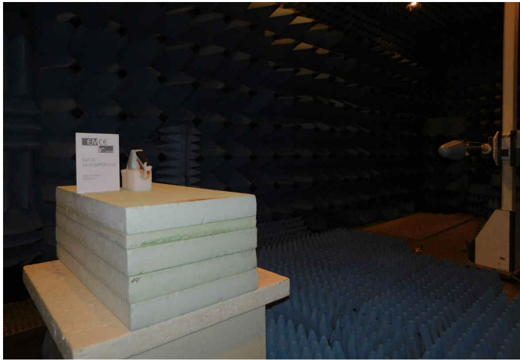
Test setup – SAC [1 – 10 GHz]
