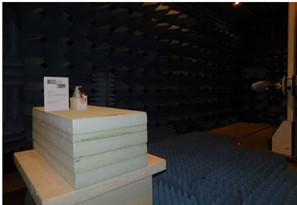
Final test setup – SAC [1 – 10 GHz]
