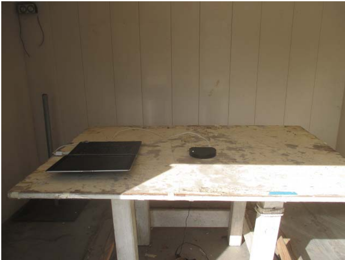
Figure 1 EUT Configuration for Radiated Emission Test
