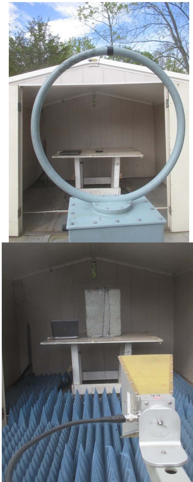
Figure 2 Radiated Emission Test Setup
