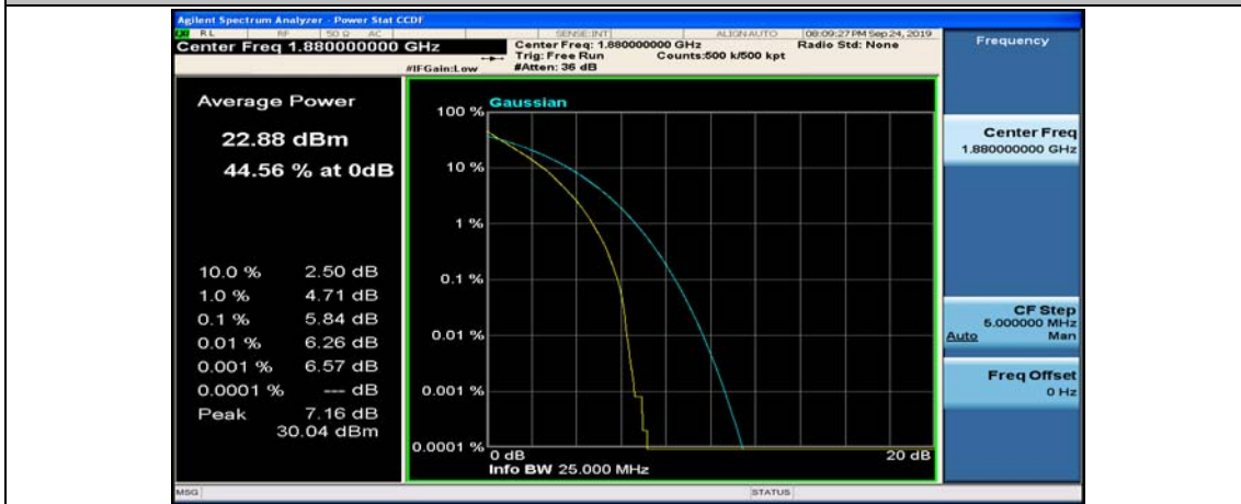
(Channel Bandwidth:15 MHz)_MCH_QPSK_75RB#0
