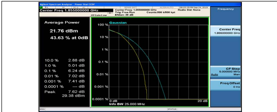
Channel Bandwidth: 10 MHz_MCH_16QAM_1RB#0
