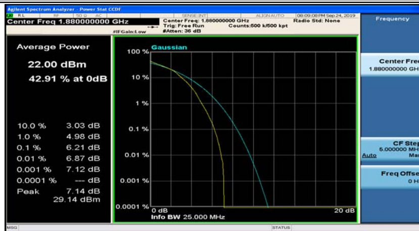
(Channel Bandwidth:15 MHz)_MCH_16QAM_37RB#18
