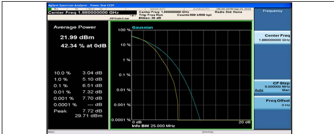
(Channel Bandwidth:15 MHz)_MCH_16QAM_75RB#0
