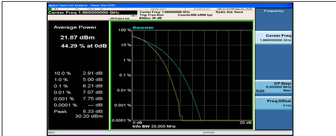
(Channel Bandwidth:20 MHz)_MCH_16QAM_1RB#0
