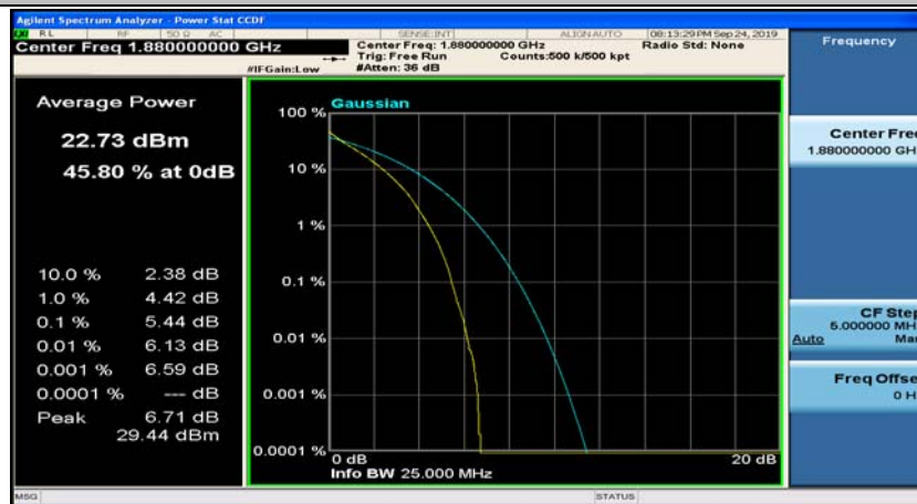
(Channel Bandwidth:20 MHz)_MCH_QPSK_50RB#25
