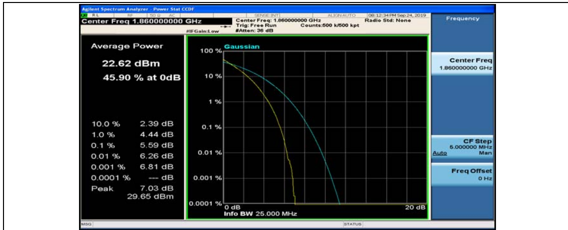
(Channel Bandwidth:20 MHz)_MCH_QPSK_1RB#0
