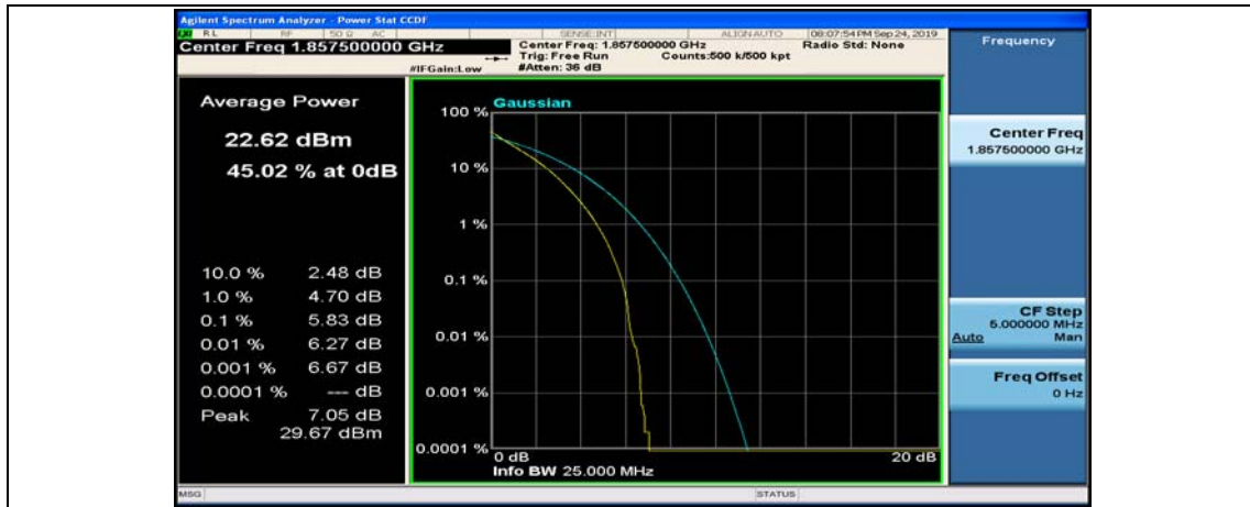
(Channel Bandwidth:15 MHz)_MCH_QPSK_1RB#0
