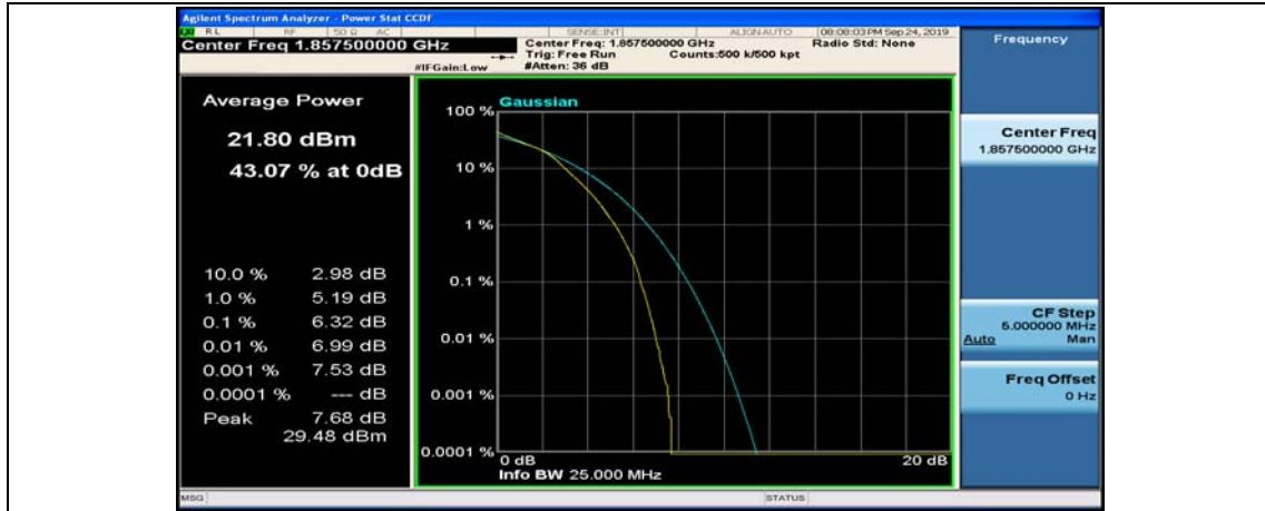
(Channel Bandwidth:15 MHz)_MCH_16QAM_1RB#0
