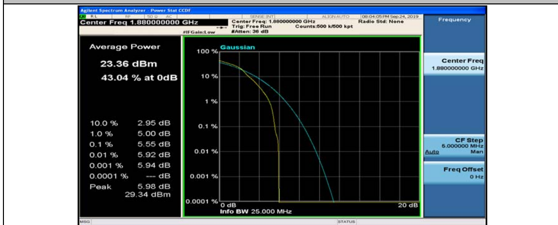
Channel Bandwidth: 10 MHz_MCH_16QAM_1RB#49
