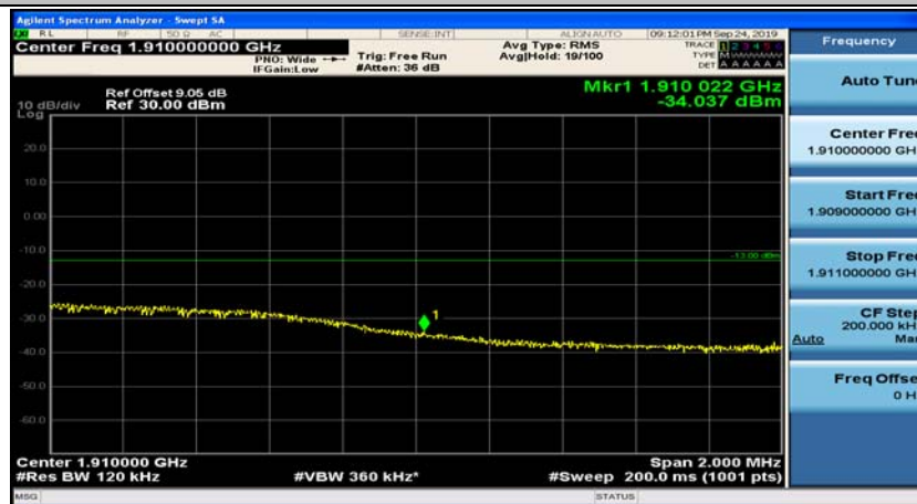
Channel Bandwidth: 10 MHz_HCH_16QAM_25RB#25
