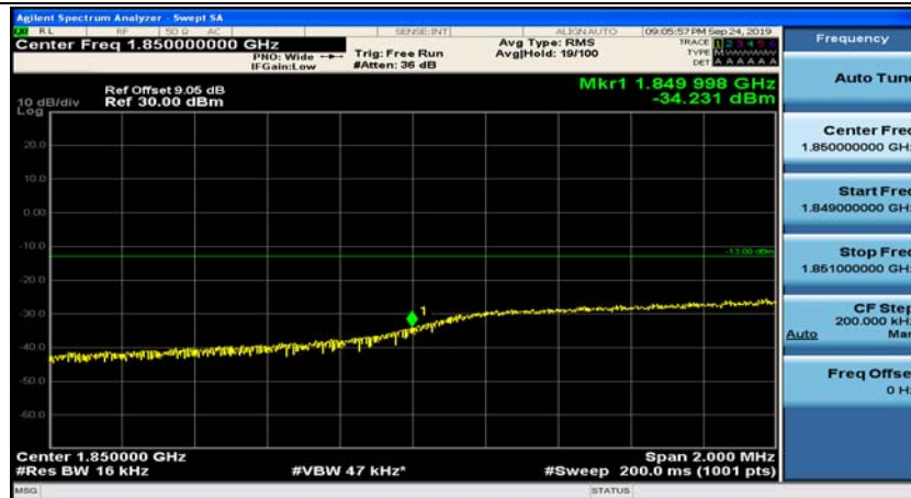
(Channel Bandwidth: 5 MHz)_LCH_QPSK_1RB#24
