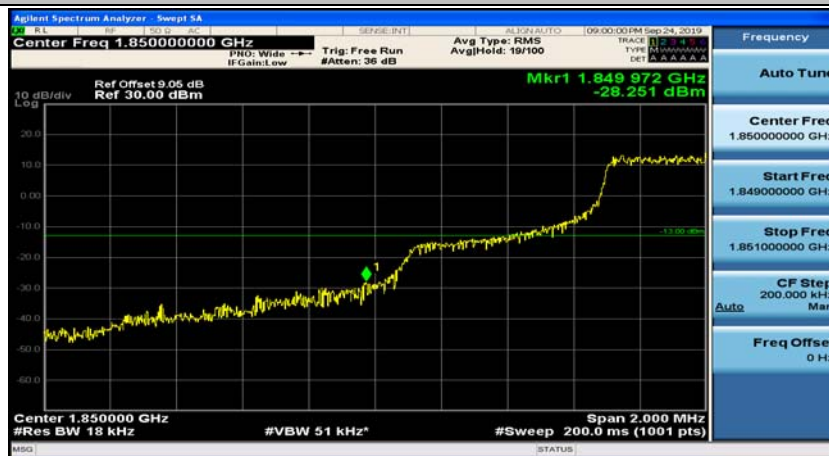
(Channel Bandwidth: 1.4 MHz)_LCH_QPSK_6RB#0
