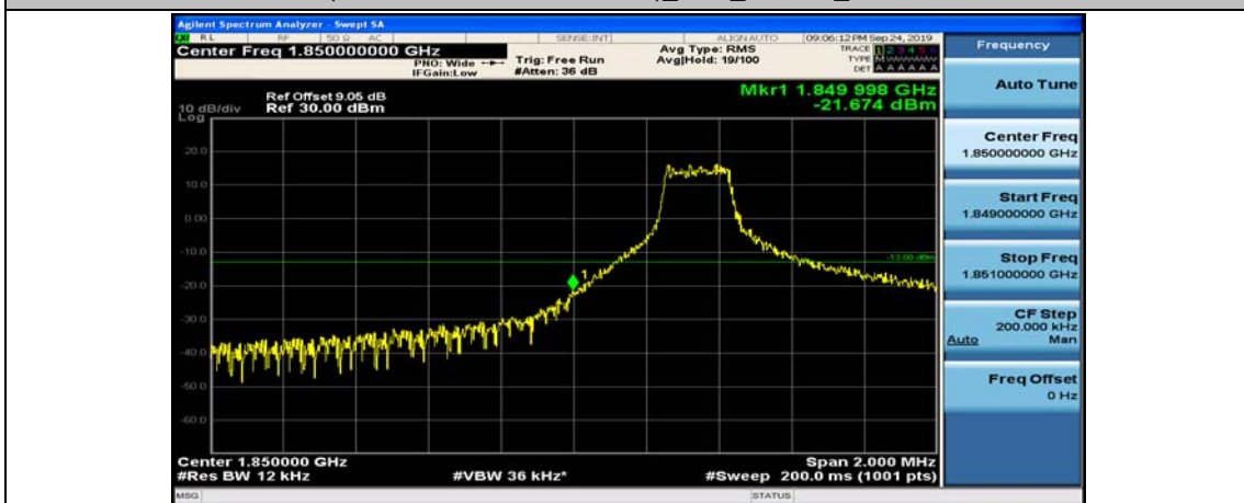
(Channel Bandwidth: 5 MHz)_LCH_16QAM_1RB#12
