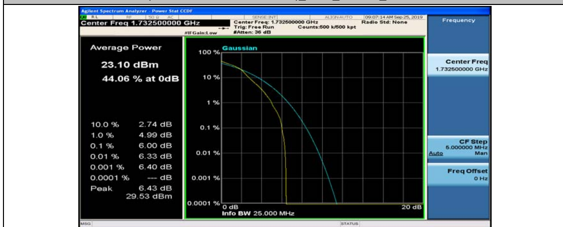
(Channel Bandwidth: 5 MHz)_MCH_16QAM_1RB#12
