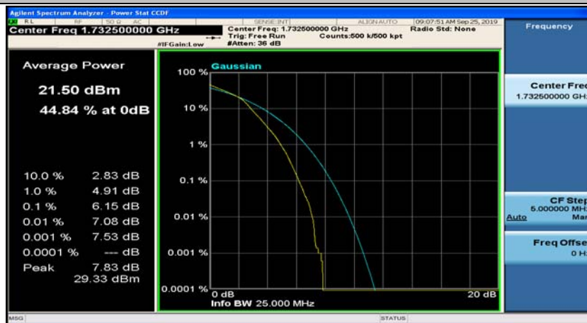
(Channel Bandwidth: 5 MHz)_MCH_16QAM_12RB#6
