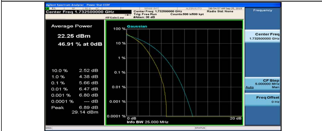
(Channel Bandwidth: 1.4 MHz)_MCH_QPSK_6RB#0
