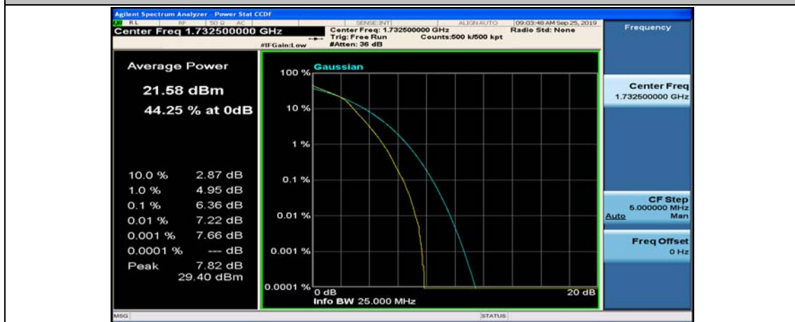
(Channel Bandwidth: 3 MHz)_MCH_16QAM_15RB#0
