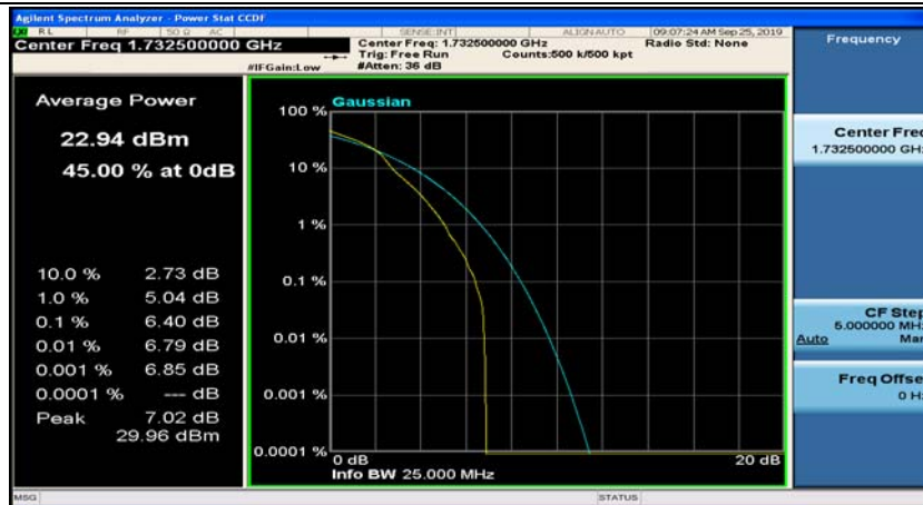
(Channel Bandwidth: 5 MHz)_MCH_16QAM_12RB#0
