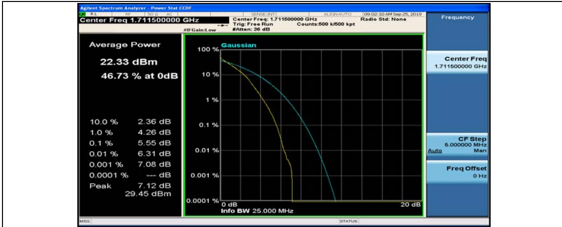
(Channel Bandwidth: 3 MHz)_MCH_QPSK_1RB#0
