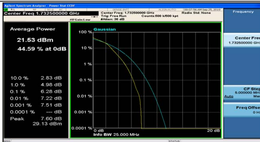
(Channel Bandwidth: 5 MHz)_MCH_16QAM_12RB#13
