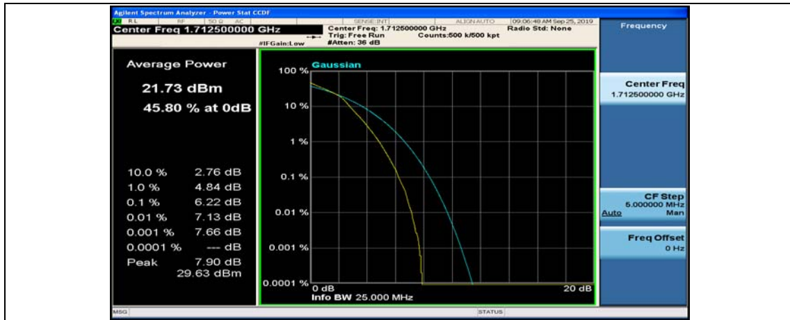
(Channel Bandwidth: 5 MHz)_MCH_16QAM_1RB#0
