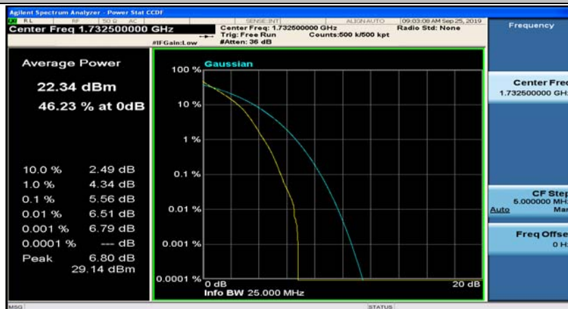
(Channel Bandwidth: 3 MHz)_MCH_QPSK_8RB#7
