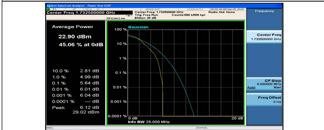
(Channel Bandwidth: 3 MHz)_MCH_16QAM_1RB#14
