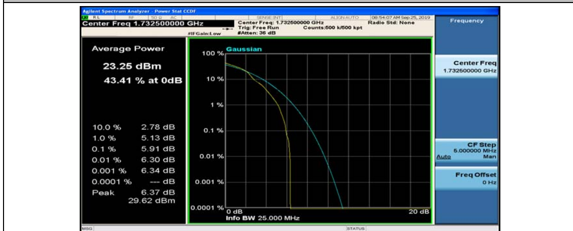
(Channel Bandwidth: 1.4 MHz)_MCH_16QAM_1RB#5
