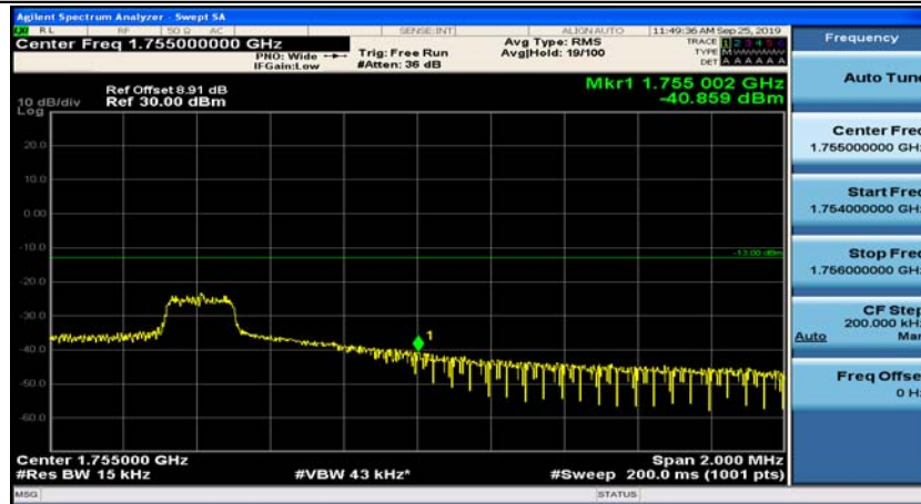
Channel Bandwidth: 10 MHz_HCH_16QAM_1RB#24
