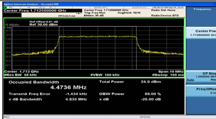
(Channel Bandwidth: 5 MHz)_LCH_QPSK_25RB#0
