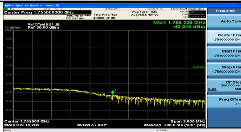
Channel Bandwidth: 10 MHz_HCH_16QAM_1RB#49
