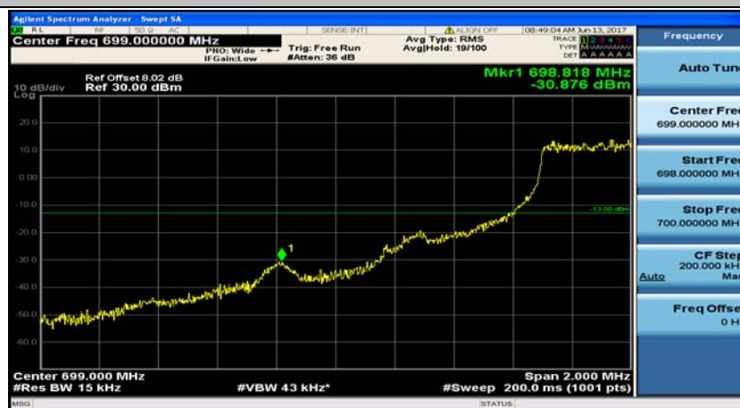
(Channel Bandwidth: 1.4 MHz)_LCH_QPSK_6RB#0
