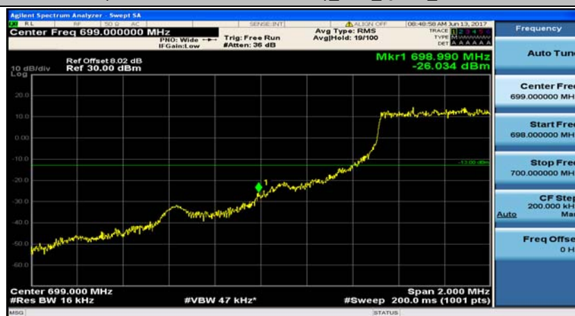
(Channel Bandwidth: 1.4 MHz)_LCH_QPSK_3RB#3
