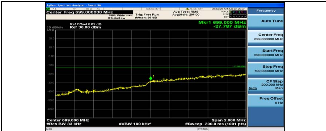
(Channel Bandwidth: 3 MHz)_LCH_QPSK_15RB#0
