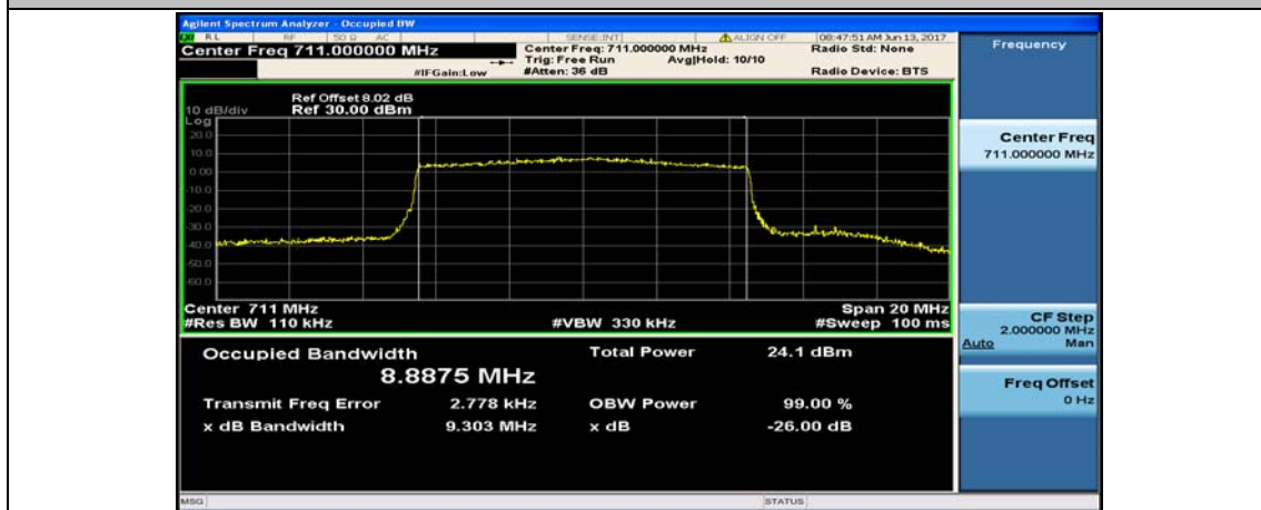
Channel Bandwidth: 10 MHz_HCH_16QAM_50RB#0
