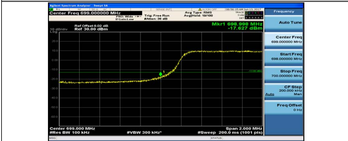
(Channel Bandwidth: 5 MHz)_LCH_QPSK_25RB#0
