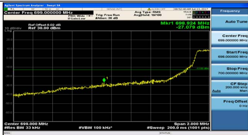
(Channel Bandwidth: 3 MHz)_LCH_16QAM_8RB#7
