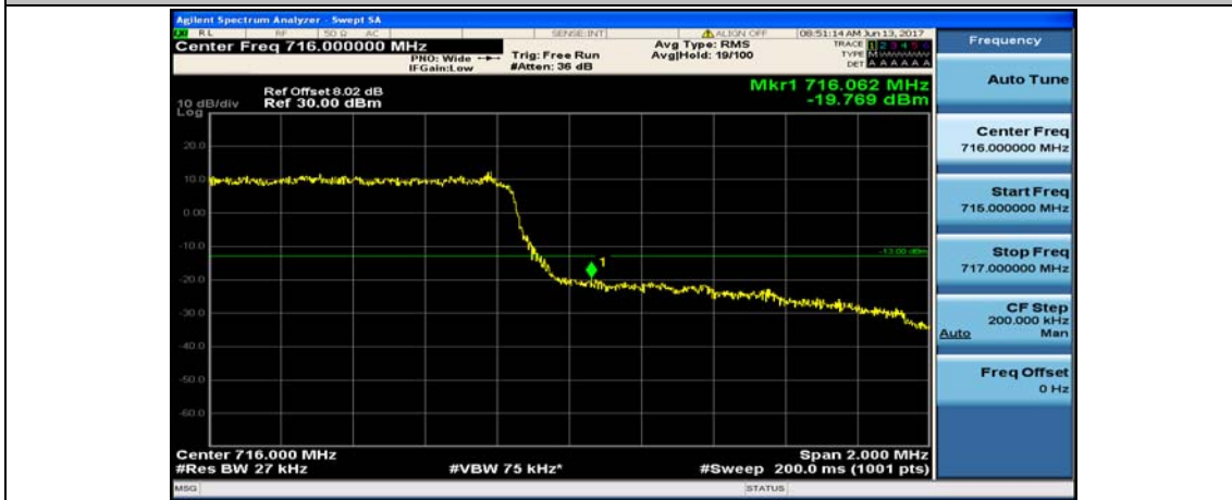
(Channel Bandwidth: 1.4 MHz)_HCH_QPSK_6RB#0
