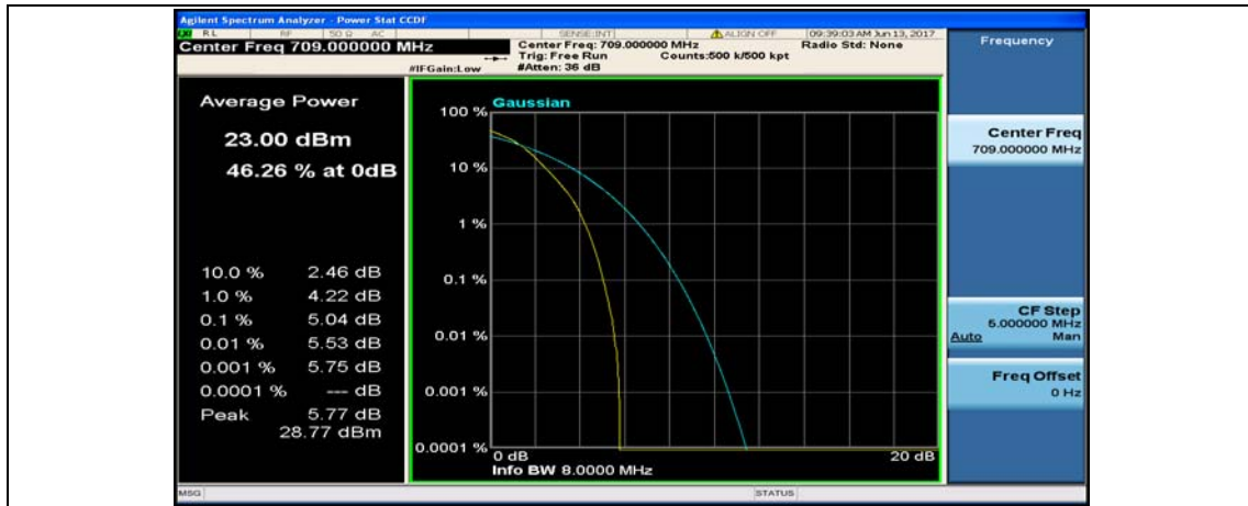
Channel Bandwidth: 10 MHz_MCH_QPSK_1RB#0
