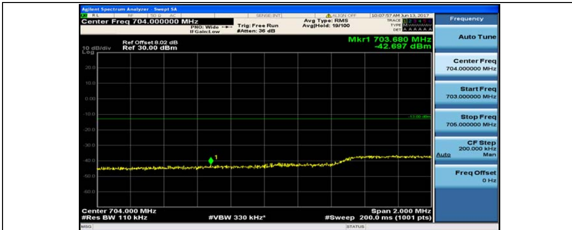
Channel Bandwidth: 10 MHz_LCH_QPSK_50RB#0
