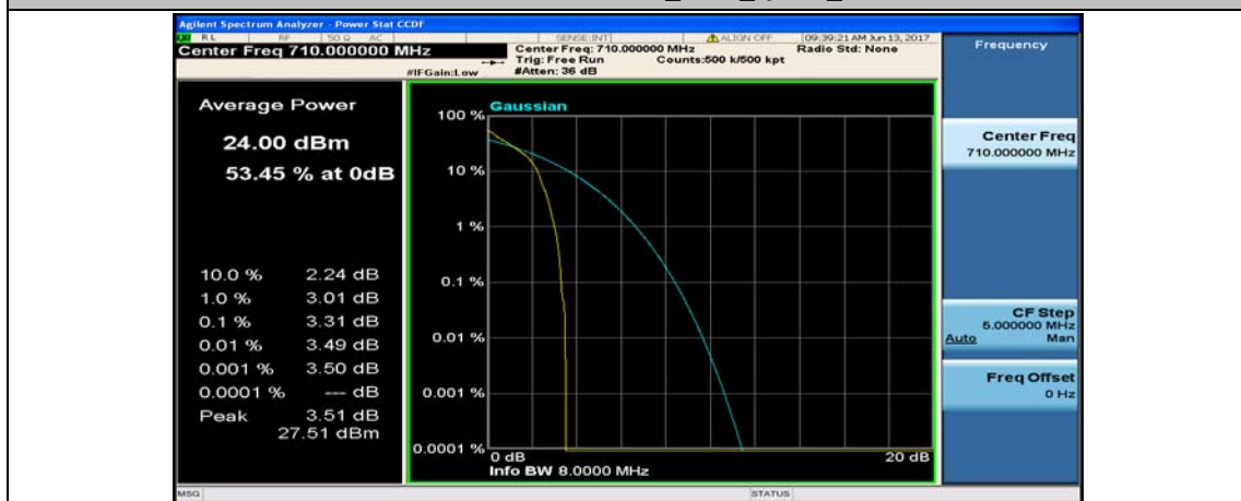
Channel Bandwidth: 10 MHz_MCH_QPSK_1RB#24
