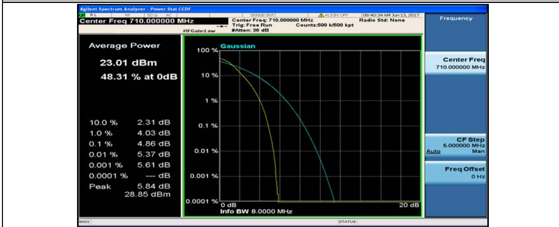
Channel Bandwidth: 10 MHz_MCH_QPSK_50RB#0
