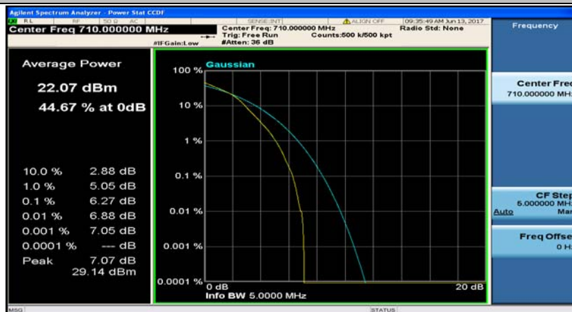
(Channel Bandwidth: 5 MHz)_MCH_16QAM_12RB#13
