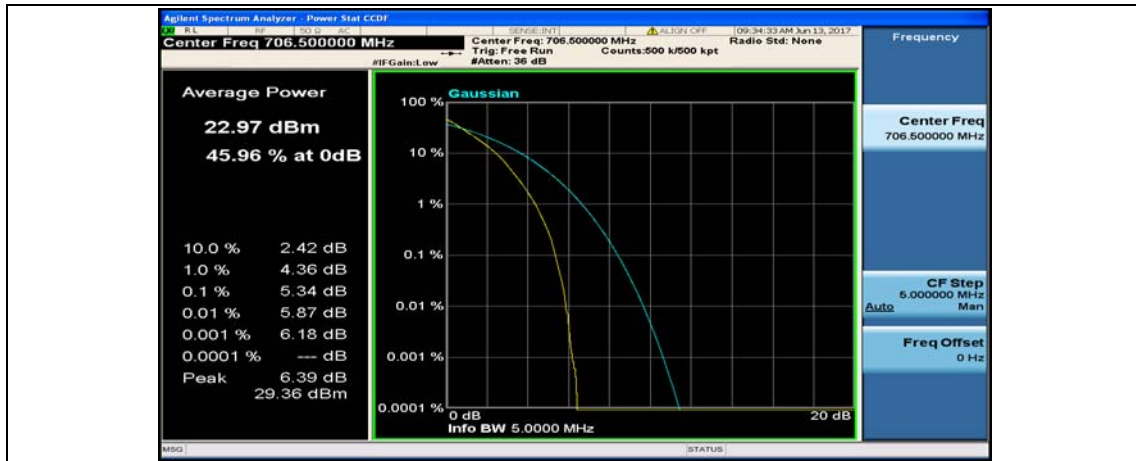
(Channel Bandwidth: 5 MHz)_MCH_QPSK_1RB#0
