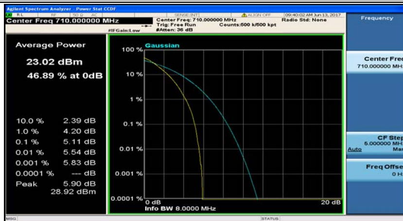
Channel Bandwidth: 10 MHz_MCH_QPSK_25RB#25
