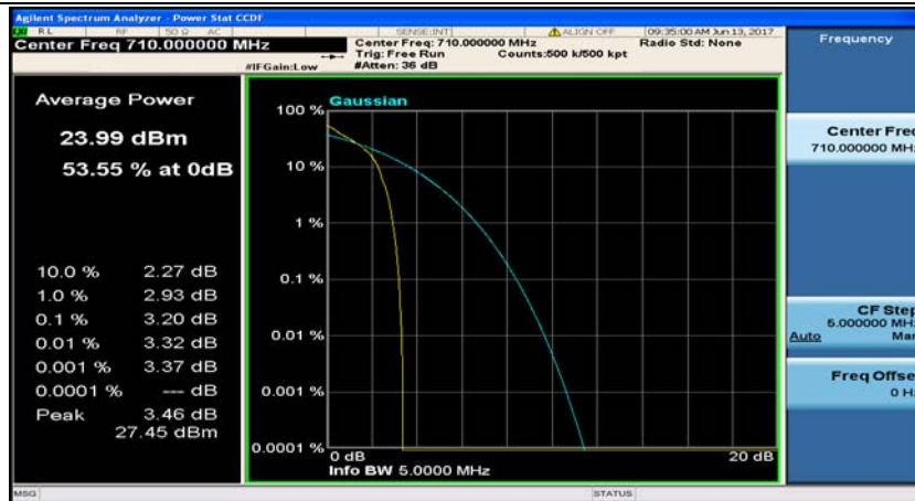
(Channel Bandwidth: 5 MHz)_MCH_QPSK_12RB#0
