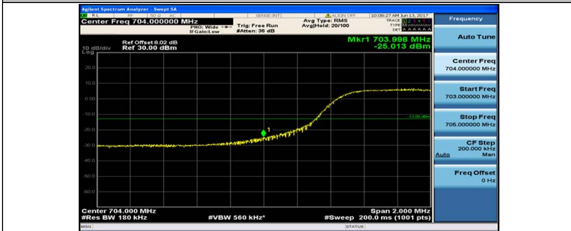
Channel Bandwidth: 10 MHz_LCH_QPSK_50RB#0
