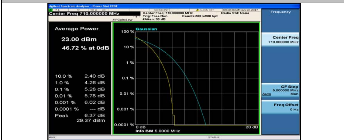
(Channel Bandwidth: 5 MHz)_MCH_QPSK_25RB#0
