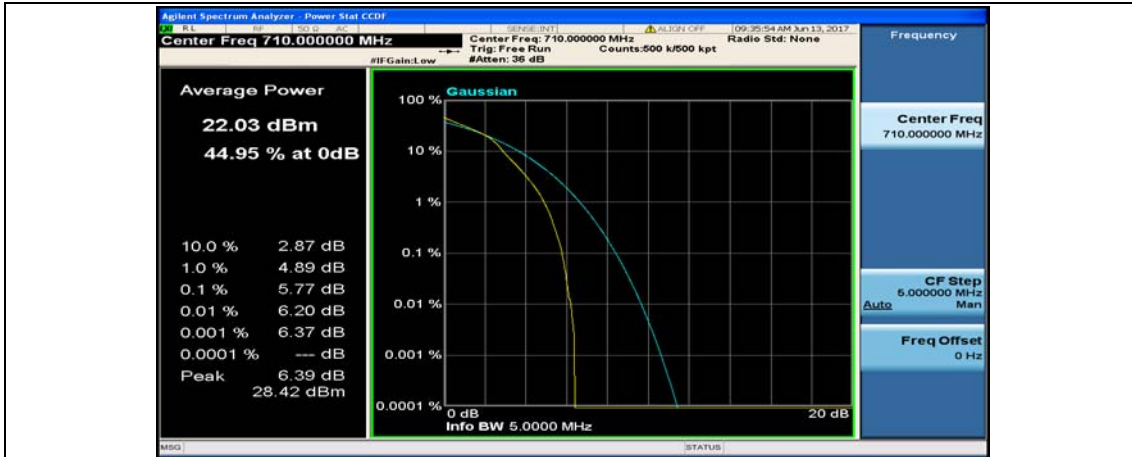
(Channel Bandwidth: 5 MHz)_MCH_16QAM_25RB#0
