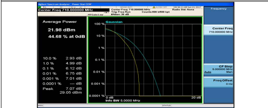
(Channel Bandwidth: 5 MHz)_MCH_16QAM_25RB#0
