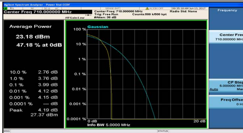
(Channel Bandwidth: 5 MHz)_MCH_16QAM_12RB#0
