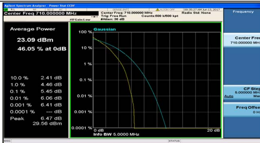
(Channel Bandwidth: 5 MHz)_MCH_QPSK_12RB#6
