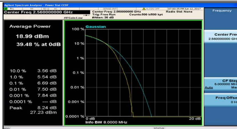
(Channel Bandwidth:20 MHz)_HCH_16QAM_100RB#0
