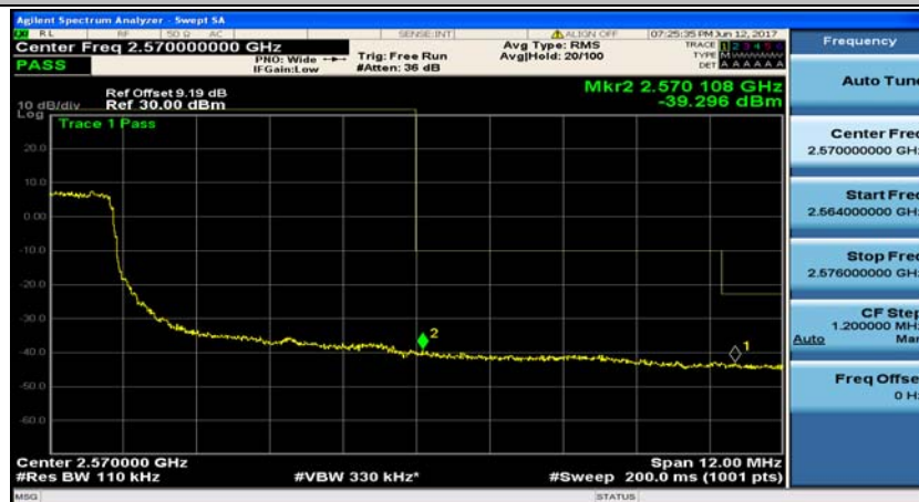
Channel Bandwidth: 10 MHz_HCH_QPSK_25RB#12
