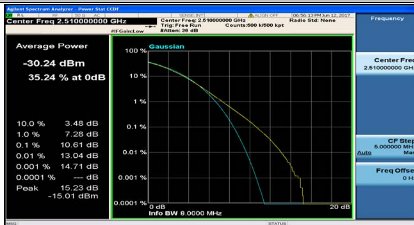
(Channel Bandwidth:20 MHz)_LCH_16QAM_50RB#0
