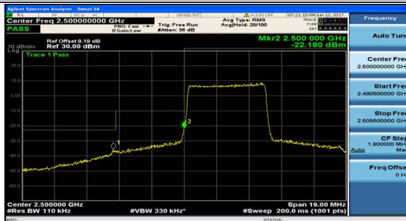
(Channel Bandwidth: 5 MHz)_LCH_16QAM_25RB#0
