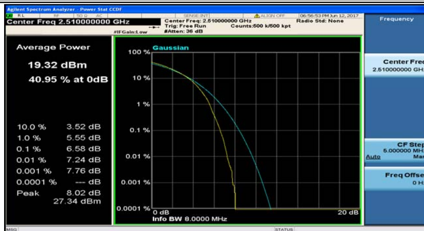
(Channel Bandwidth:20 MHz)_LCH_16QAM_100RB#0
