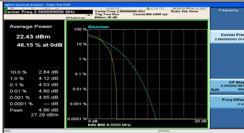
(Channel Bandwidth:20 MHz)_HCH_16QAM_1RB#99
