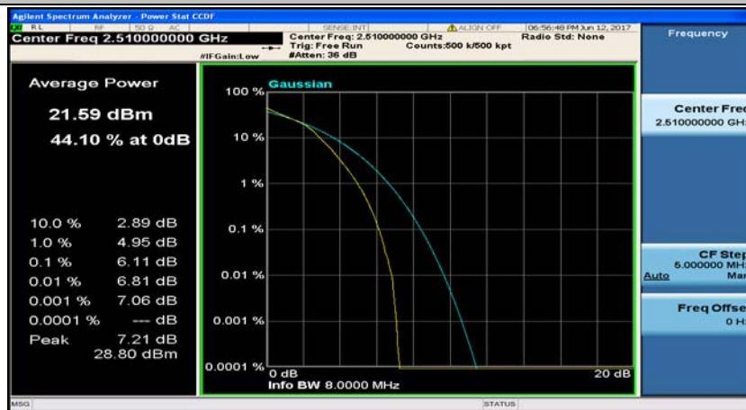
(Channel Bandwidth:20 MHz)_LCH_16QAM_50RB#50
