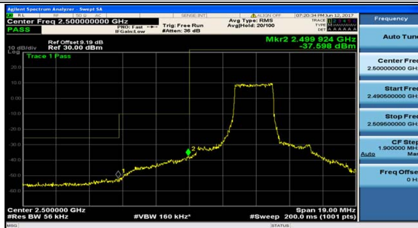
(Channel Bandwidth: 5 MHz)_LCH_QPSK_25RB#0
