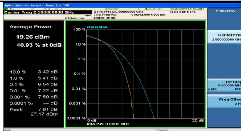
(Channel Bandwidth:20 MHz)_HCH_16QAM_50RB#25
