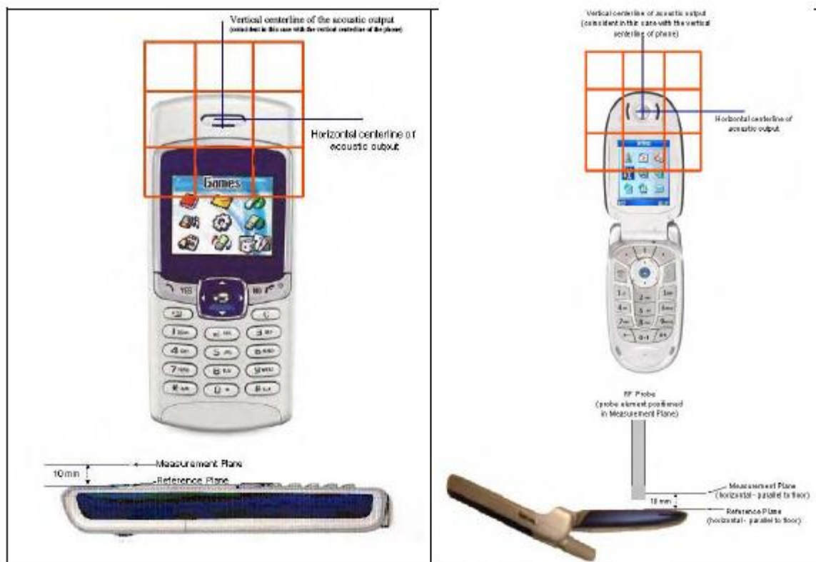
Reference and plane for RF emission measurements
