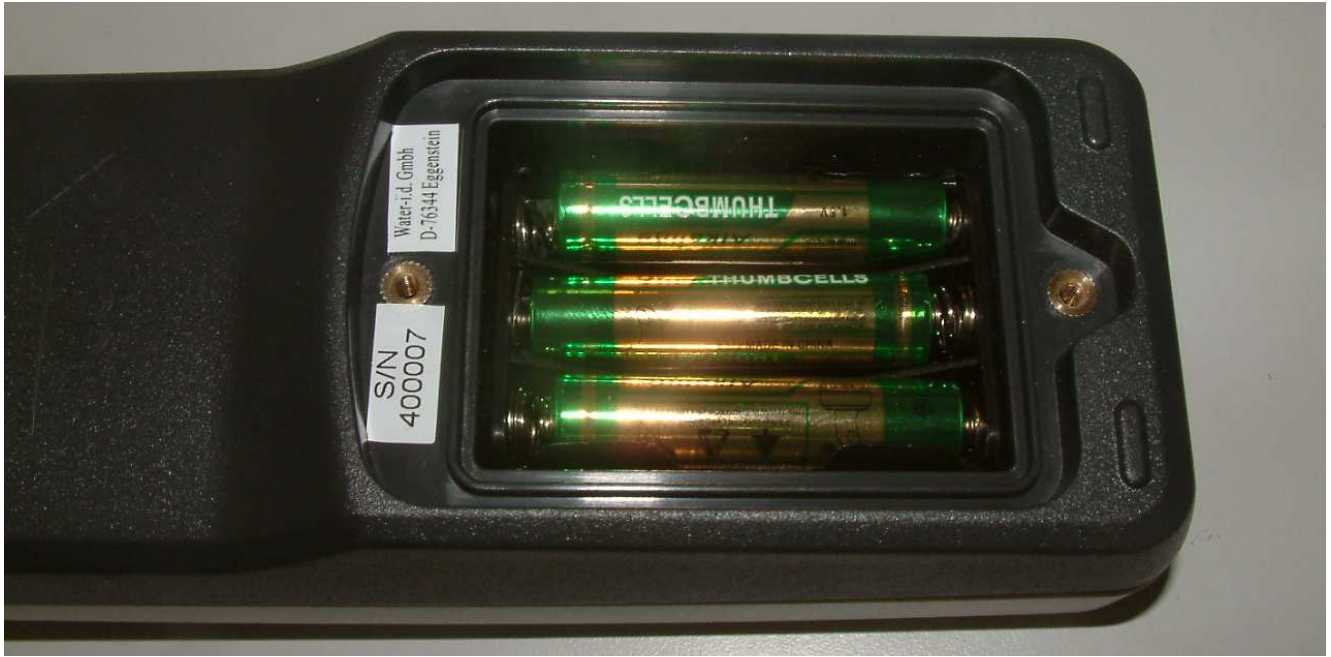
Battery cover removed
