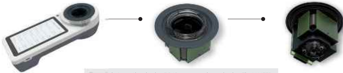
The built-in SmartChamber has 3 PCBs, connected to each other. The MASTER PCB receives LED signals from either 180° (direct) or 90° (indirect), required for NTU-Turbidity and water samples which need to be excited, such as for PTSA, Fluorescein or Plankton.
