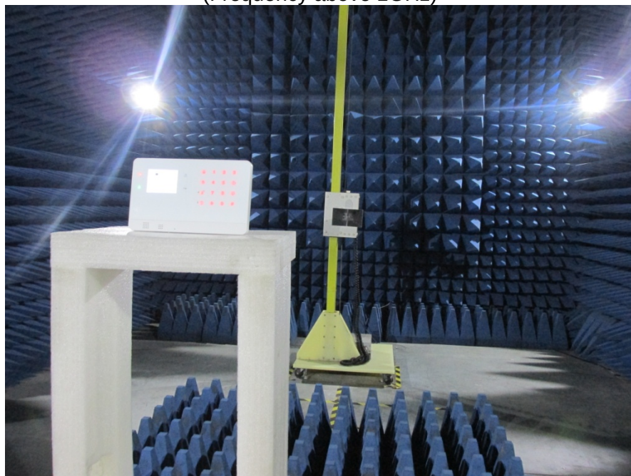
RADIATED EMISSION TEST (Frequency above 1GHz)
