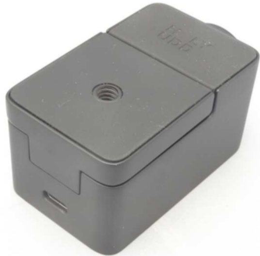
EUT, showing rear side with USB type-C connector J2 and bottom side with metal foot (metal foot can be angled, e.g. to clip the camera to a laptop screen)
