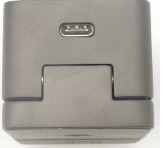
Rear side with USB Type-C connector J2
