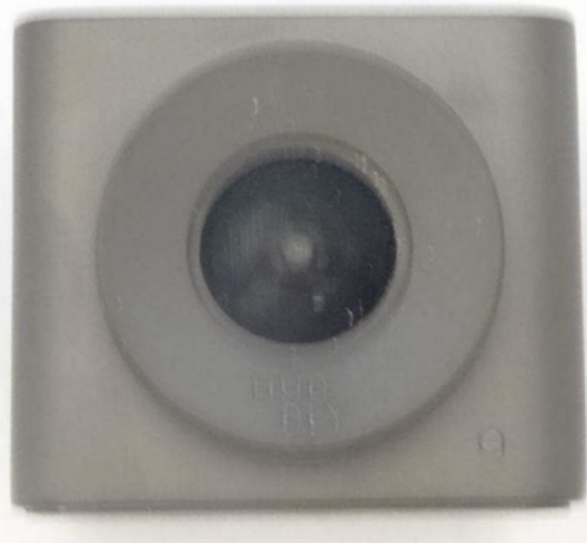
Front side with camera lens and indicator light (bottom right)
