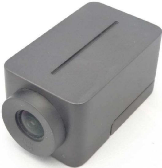
EUT, showing front side with camera lens and top side with slot for microphone
