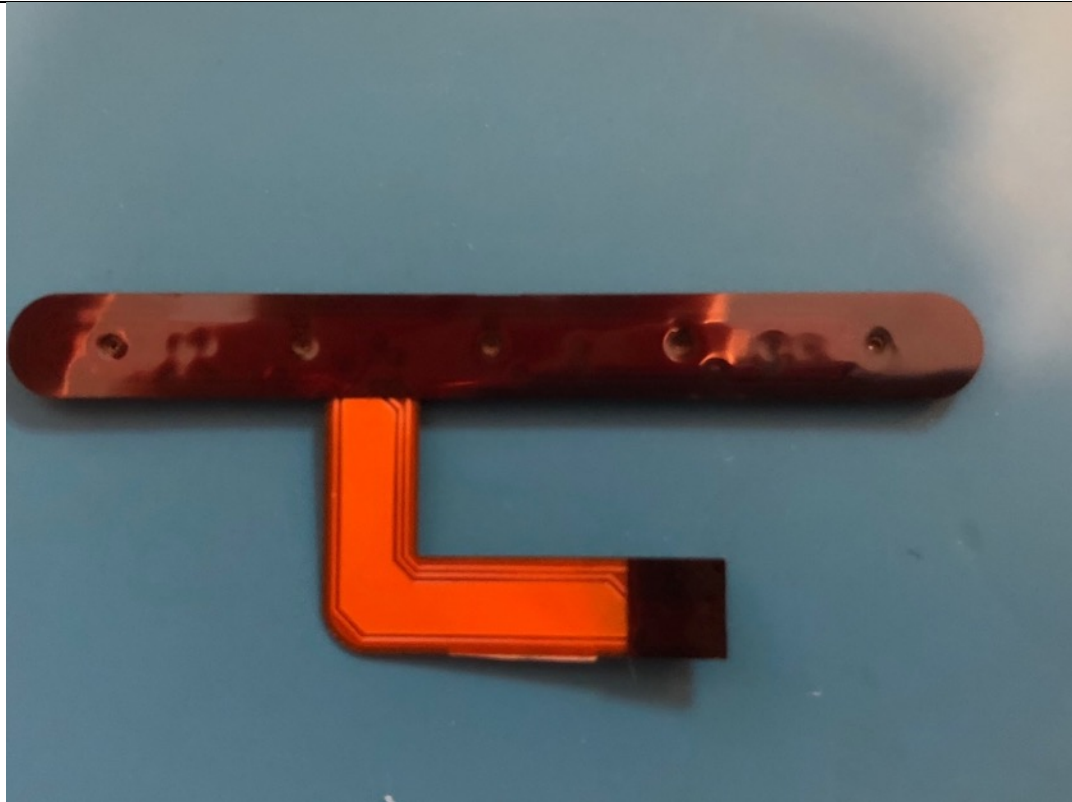
Bottom side of microphone array FPC
