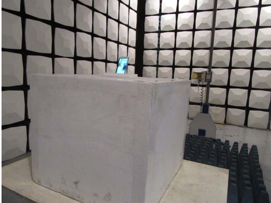
Radiated Emission View (Above 1GHz)
