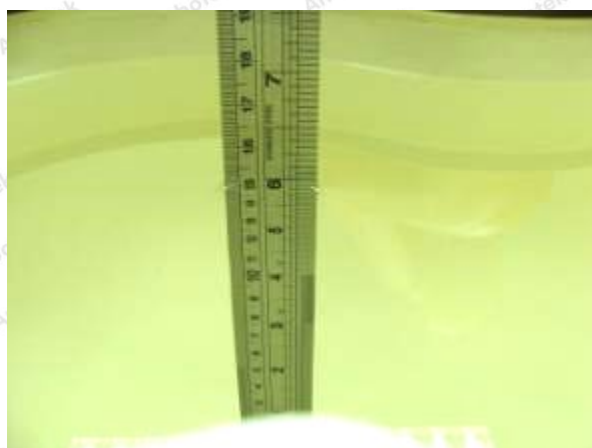
Photo of Liquid Height for Head SAR
