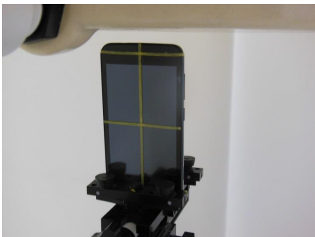
Top Side, Test Separation 10 mm
