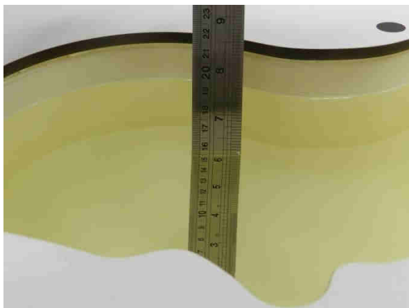
Fig 10.1 Photo of Liquid Height for Head SAR
