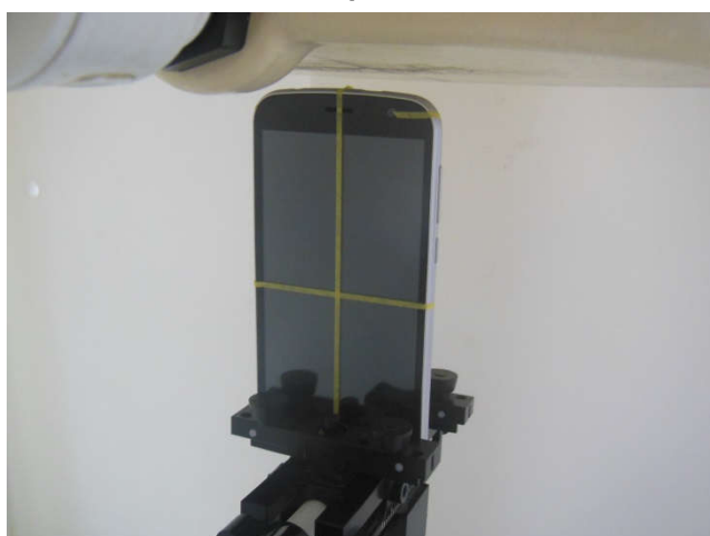
Top Side, Test Separation 10 mm
