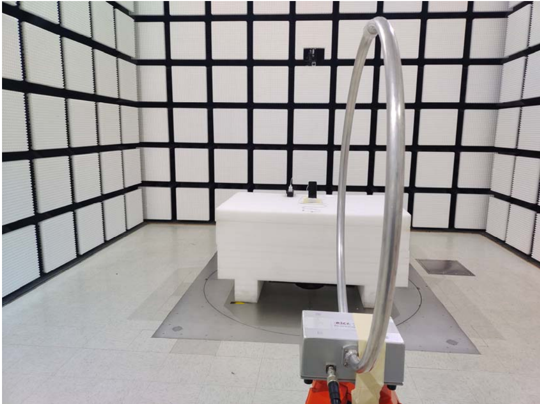
Radiated Emission 9kHz-30MHz View-Ground-parallel
