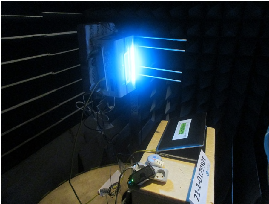
Photograph 5 : Radiated Emission > 1GHz
