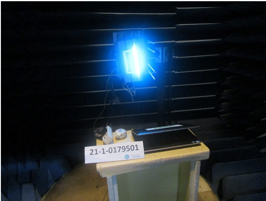
Photograph 4 : Radiated Emission > 1GHz
