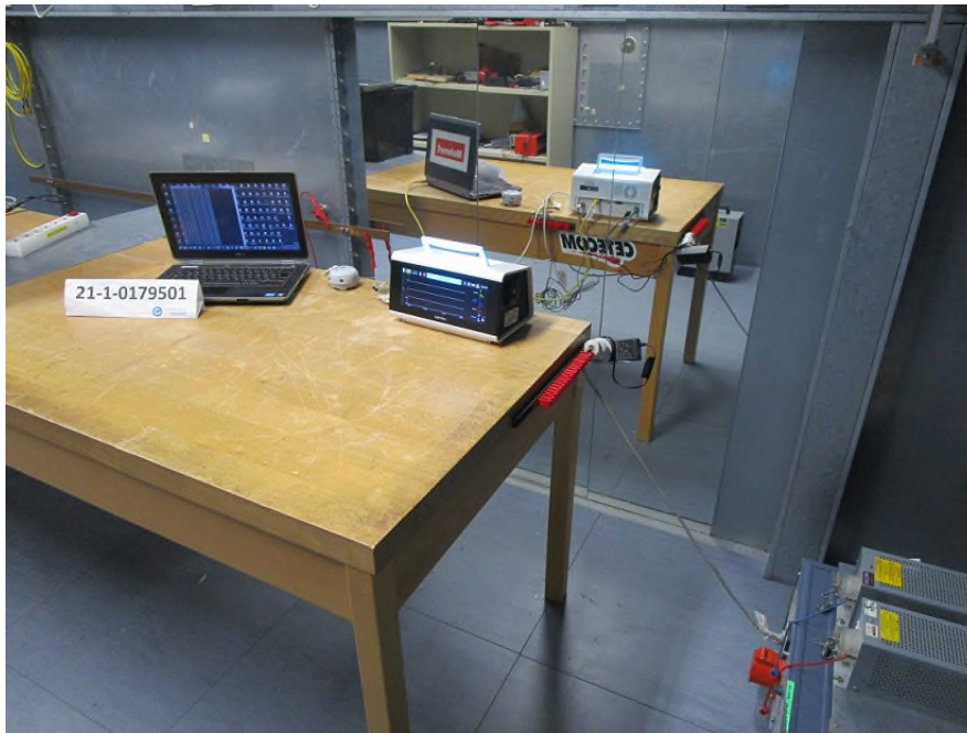
Photograph 1 : conducted Emission, test set-up
