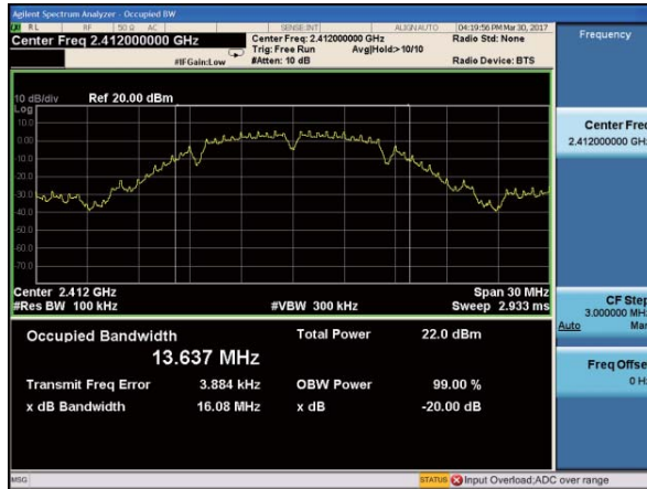
(802.11b) -20dB Bandwidth plot on channel 6
