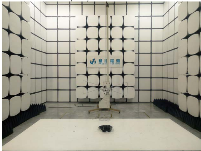
Radiated Spurious Emissions Test Frequency From 30MHz-1000MHz
