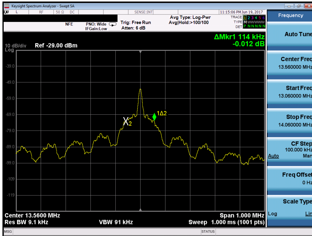
Figure 7-3. 20dB Bandwidth Plot (160143-915)
