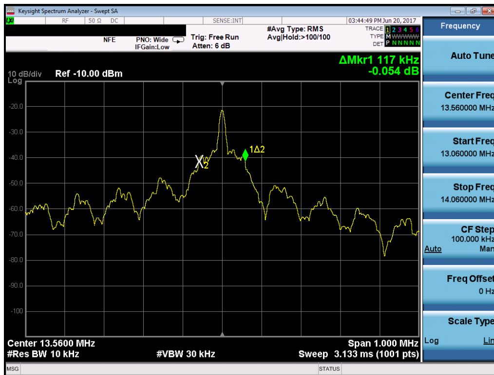
Figure 7-4. 20dB Bandwidth Plot (160132-915)
