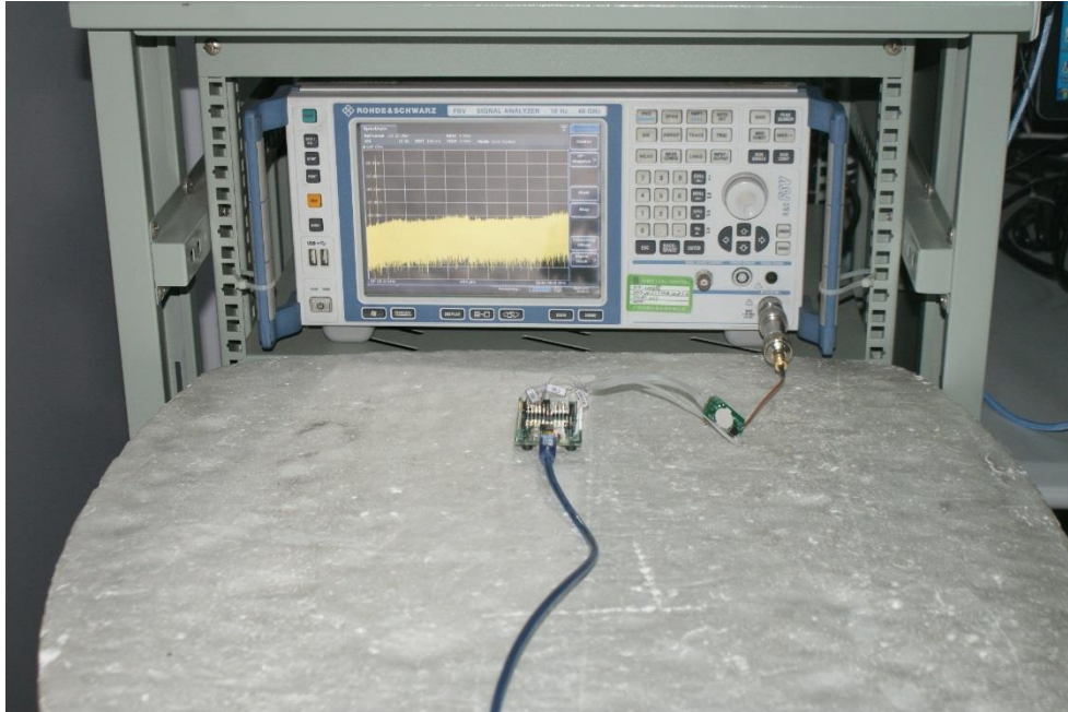
Photograph 2: Set-up for Spurious Emissions (9kHz-30MHz)
