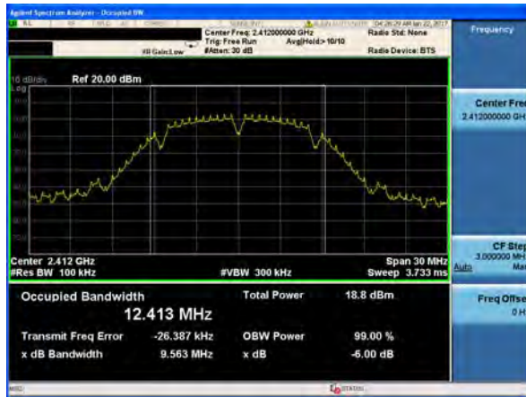
(802.11b) 6dB Bandwidth plot on channel 6
