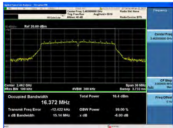
(802.11g) 6dB Bandwidth plot on channel 11
