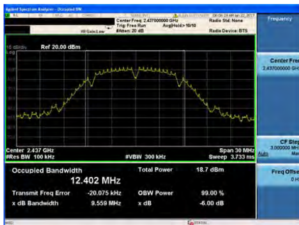
(802.11b) 6dB Bandwidth plot on channel 6
