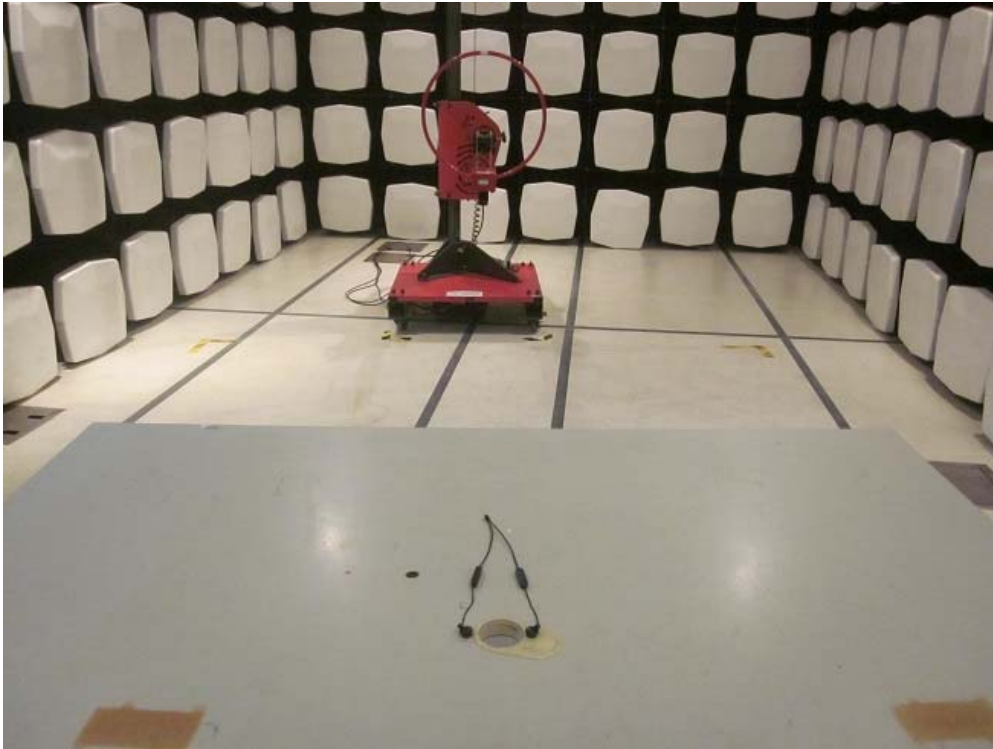
Measurement of Radiated Emission Test Set Up
