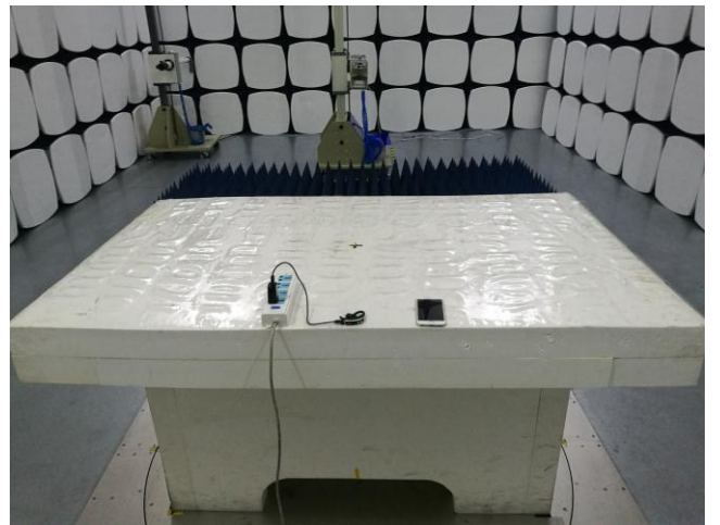
Radiated Spurious Emissions Test Setup Above 1GHz
