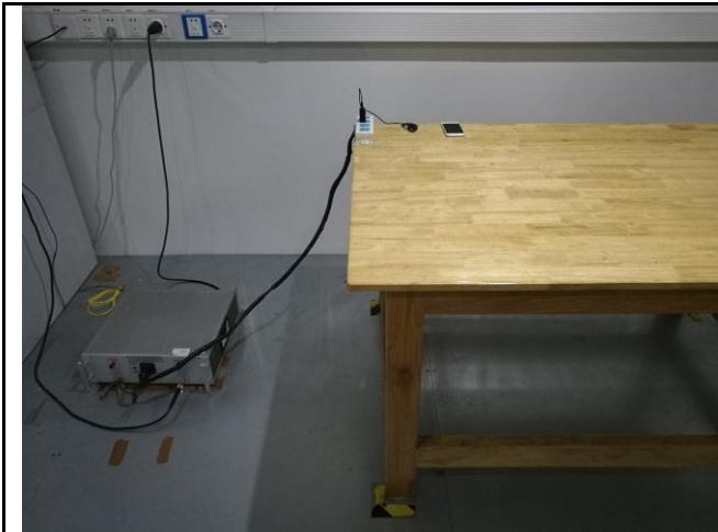
Conducted Emissions Test Setup Front View
