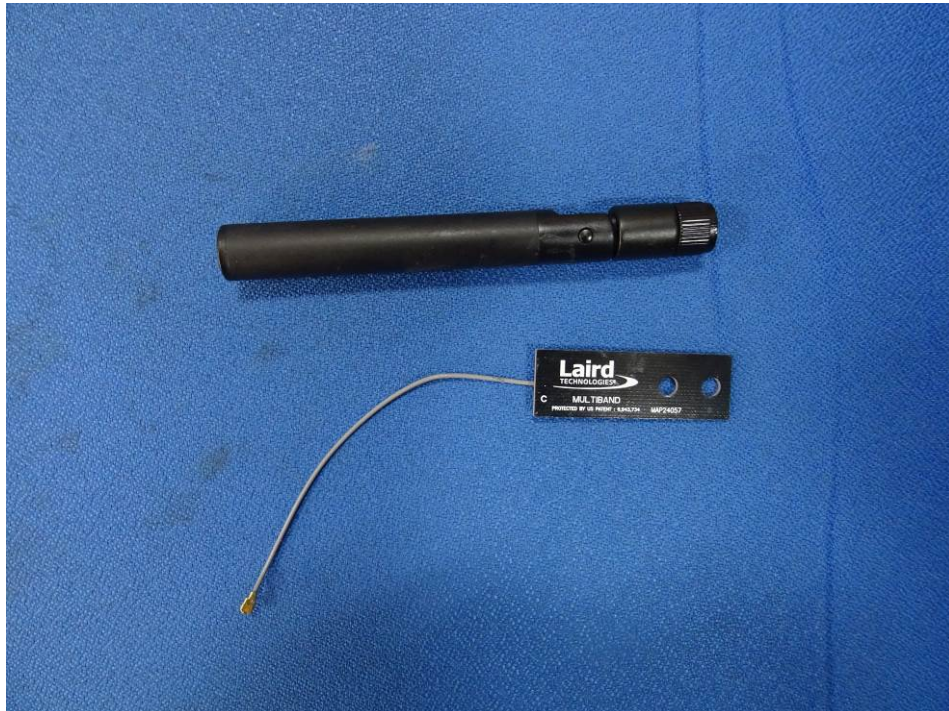
Antennas Used with RF module
