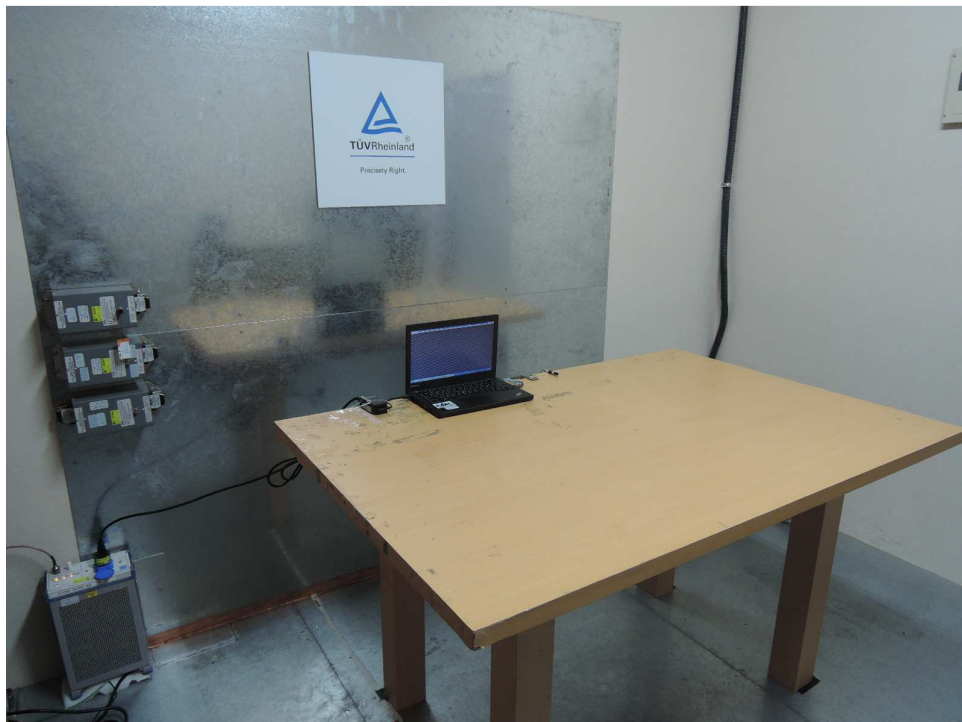
Photograph 6: Set-up for for Mains Conducted testing Front
