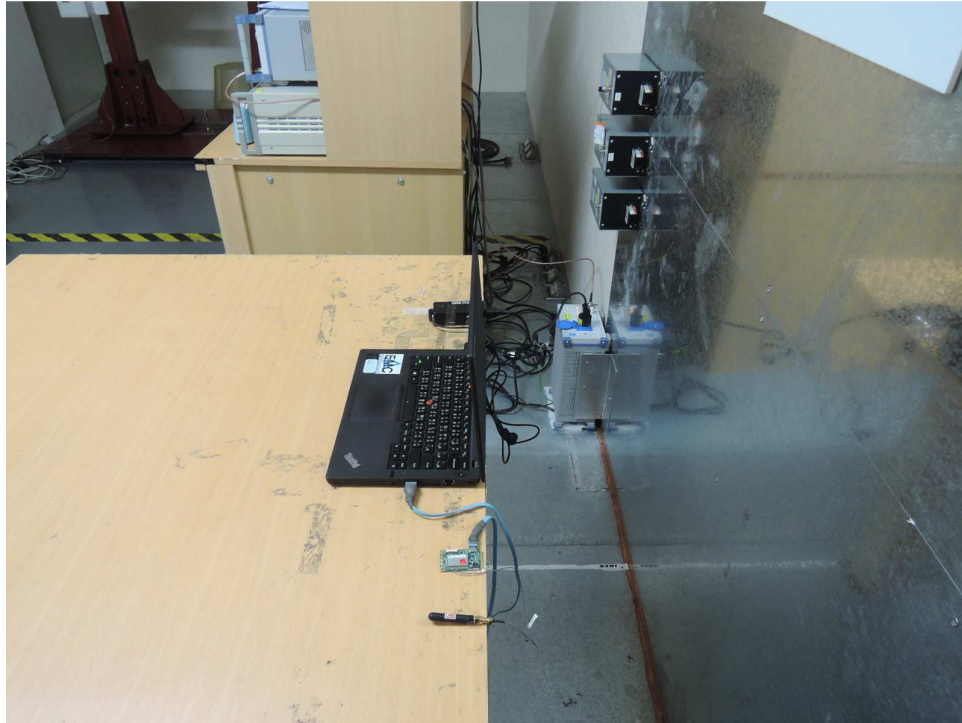
Photograph 5: Set-up for for Mains Conducted testing Back
