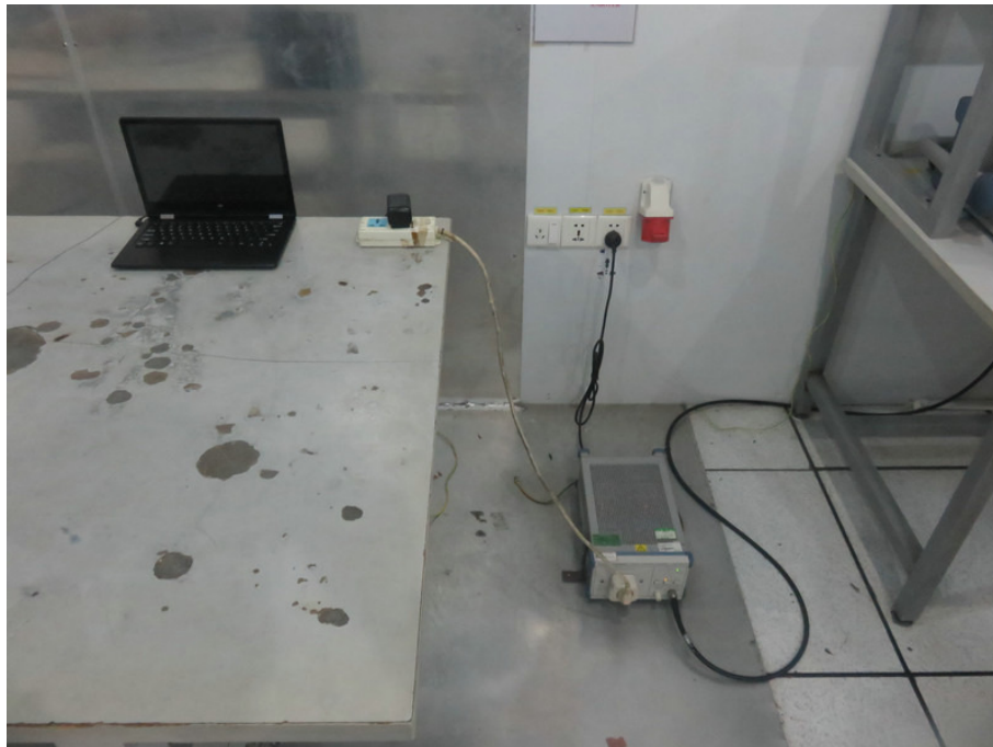
Photo of Conducted Emission Measurement
