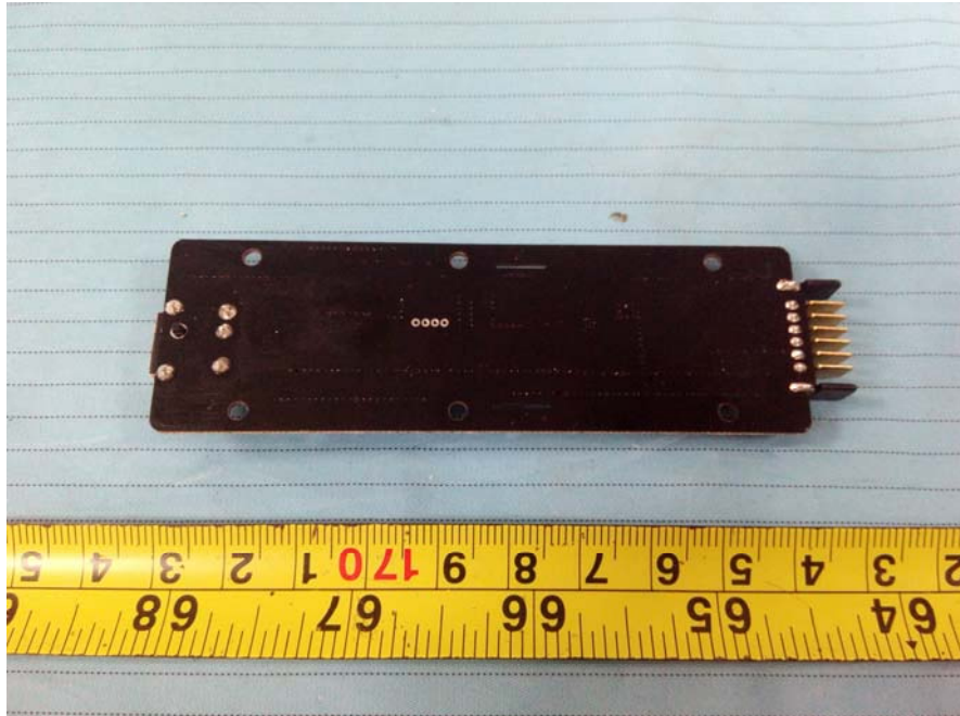
EUT – Main Board Bottom View (Battery Charger)
