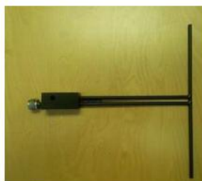
Figure 1 – MVG COMOSAR Validation Dipole
